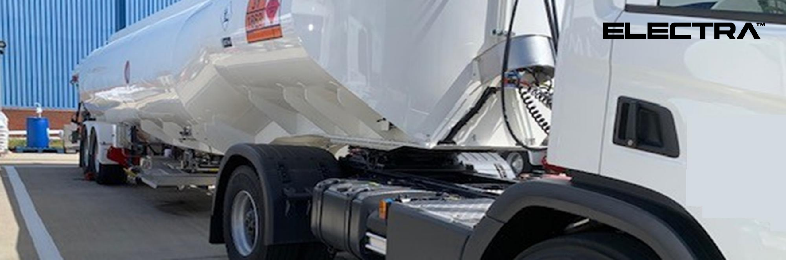
Exchange diesel chassis with Electra eStar 4x2 Tractor Unit with 210kWh battery pack
